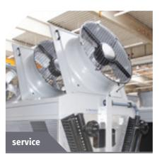
tiltable fans for the optimization of maintenance interventions on the heat exchanger
